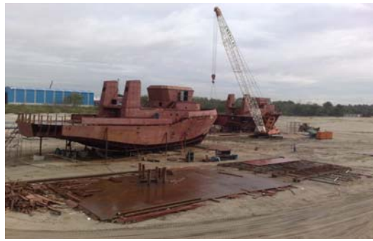
Building of 2400 HP Twin Screw Steel Tug Boat – OCEANLINE 281, 282, 283 and 285
