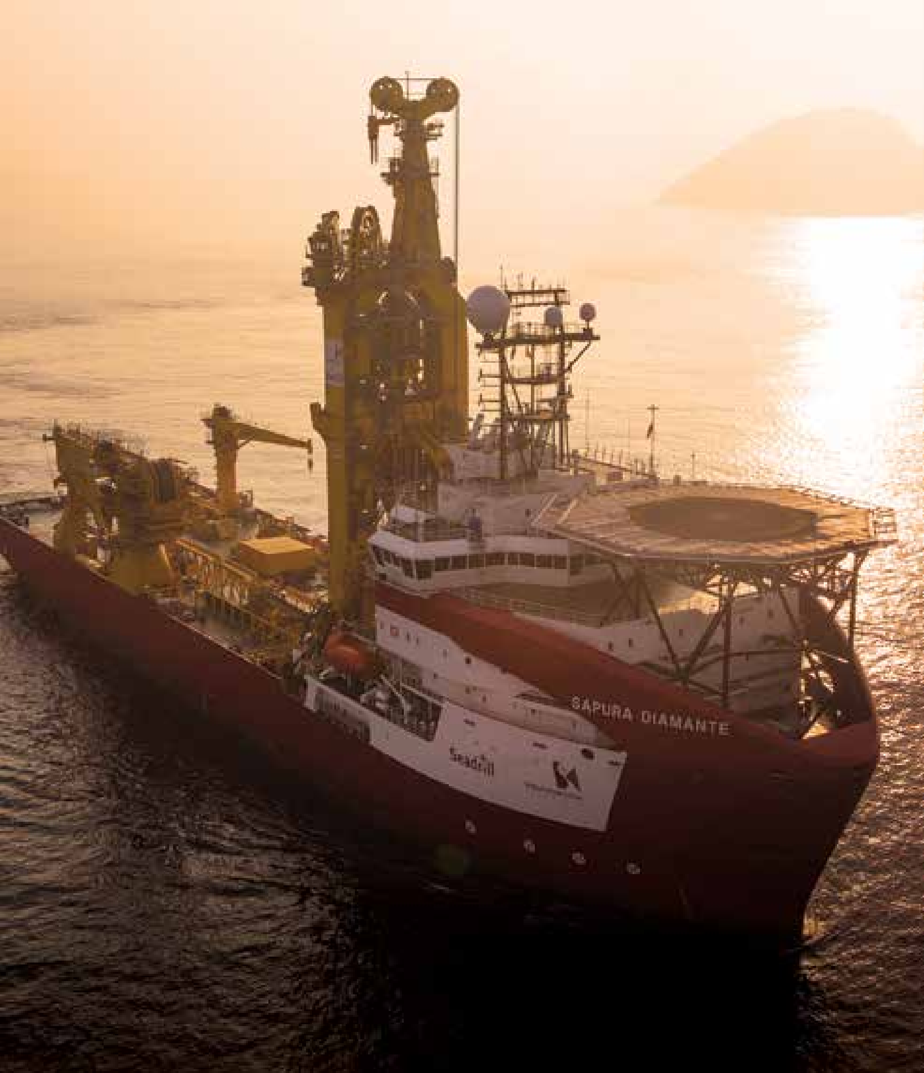
The Sapura Diamanté is the first of our fleet of six pipe-laying support vessels which will be used to develop deep-water oilfields up to 3,000 metres deep offshore Brazil for Petrobras
